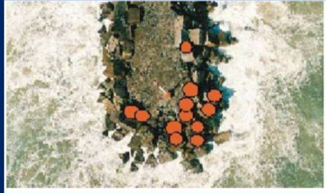
Coffs Harbour Head Storm Damage May 1997 12 x 40 tonne blocks
