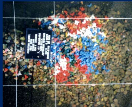
(b) Stage Two, Test 7 - extensive damage to 8 tonne Hanbars after 500 waves
